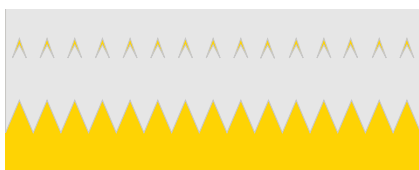
Knife bounce or high web tension.
