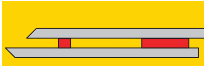
Splice tail secured with a narrow strip of PSA tape.
